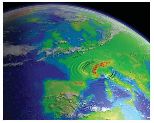
Fig. 1. Schematic visualization of the propagation of earthquake waves at the Earth's surface where the faster P and S body waves have travelled further than the Love and Rayleigh surface waves that produce much higher amplitudes.
