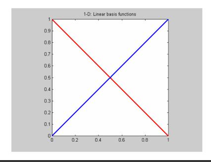
.. and  $N_{1,2}(x)$  are the linear basis functions for 1-D elements.
