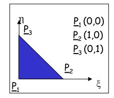
using counterclockwise numbering. Note that if  $\eta$ =0, then these equations are equivalent to the 1-D tranformations. We seek to approximate a function by the linear form
