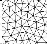
In **finite element** analysis we approximate a function defined in a Domain  $D$  with a set of orthogonal basis functions with coefficients corresponding to the functional values at some node points.
