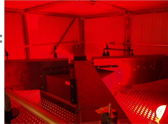
**Internal temperature is controlled by IR-lamps T: 8°C--> 13°C, relative humidity--> 60%**
