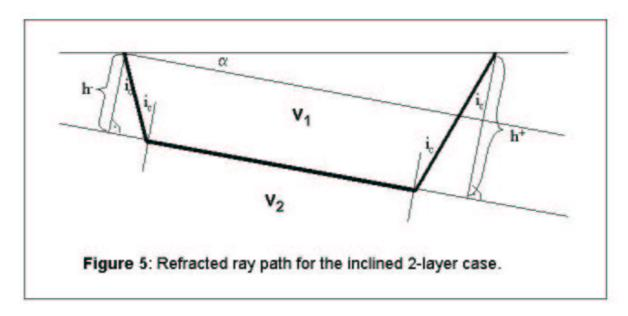
Let us develop the *forward problem*, i.e. calculating the travel times of the direct and refracted waves for a given model. With seismic velocities  $v_1$  and  $v_2$  and inclination angle  $\alpha$  the travel time of the refracted waves are
