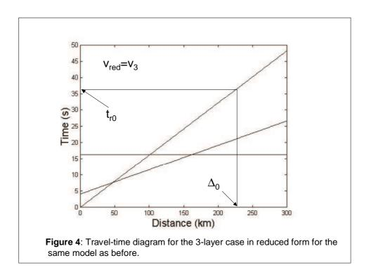
To determine he velocity-depth structure from a travel-time diagram in reduced form you can - after having calculated the *real* velocities using equation (15) - follow the steps given in section 2.3.
