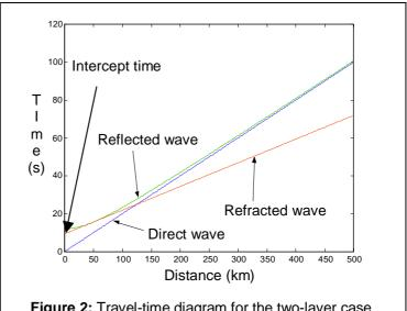
Figure 2: Travel-time diagram for the two-layer case.
