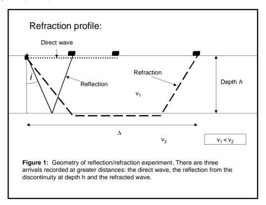
Before we try to determine the structure from observed travel times we have to understand the *forward problem*: how can we determine the travel time of the three basic rays as a function of the velocity structure and the distance from the source. The most important ingredient we need is Snell's law
