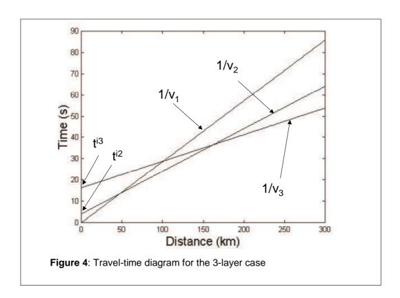
In the model shown in Figure 4 the velocites are  $v_1$ =3.5km/s,  $v_2$ =5km/s,  $v_3$ =8km/s. The layer thicknesses are  $h_1$ =10km and  $h_2$ =25km.
