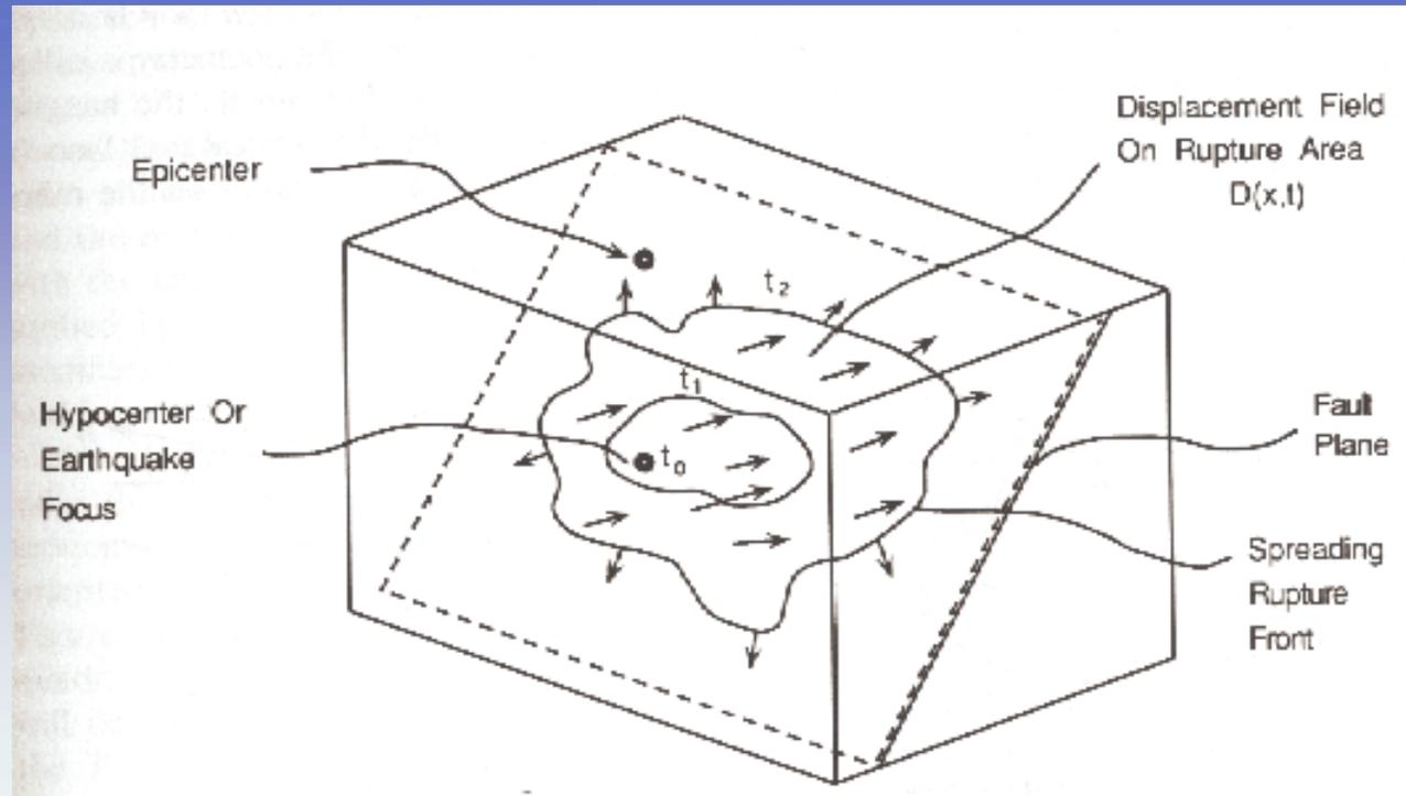
Schematic diagram of rupture on a fault. All regions sliding radiate outgoing P- and shear waves. Note that the direction of rupture propagation is not in general parallel to the slip direction.
