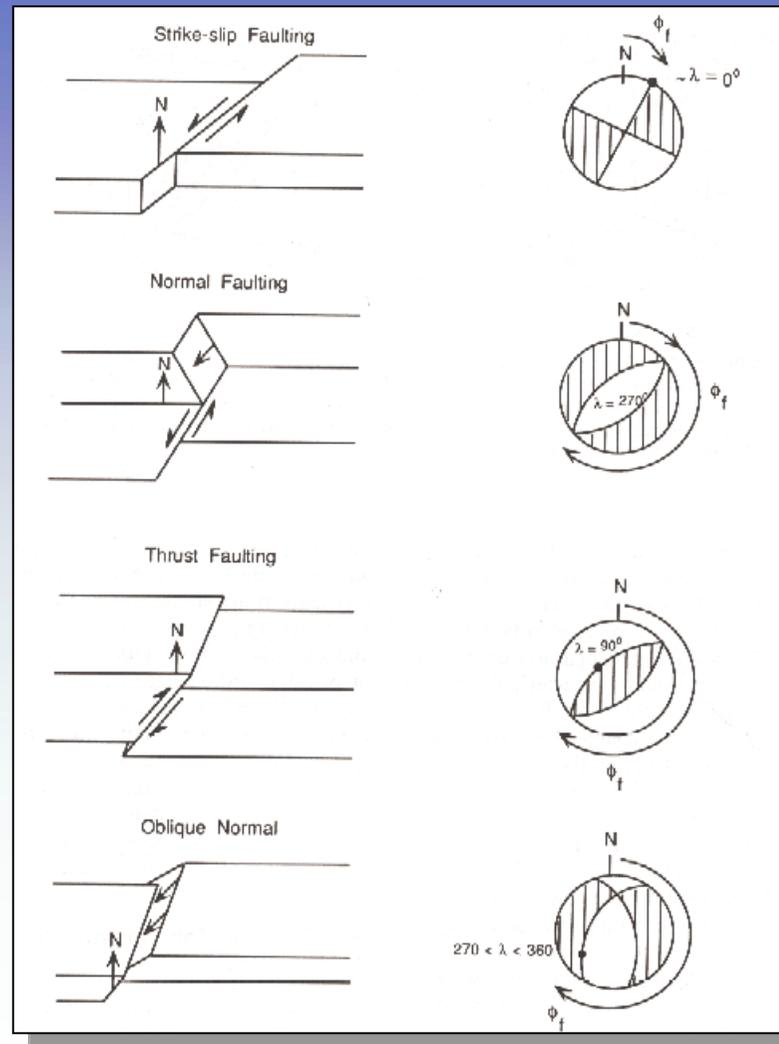
Basic fault types and their appearance in the focal mechanisms. Dark regions indicate compressional P-wave motion.
