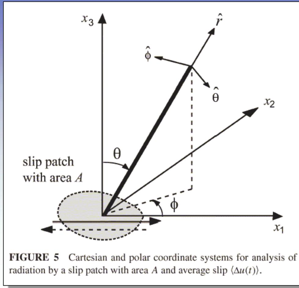
Geometry we use to express the seismic wavefield radiated by point double-couple source with area  $A$  and slip  $\Delta u$
