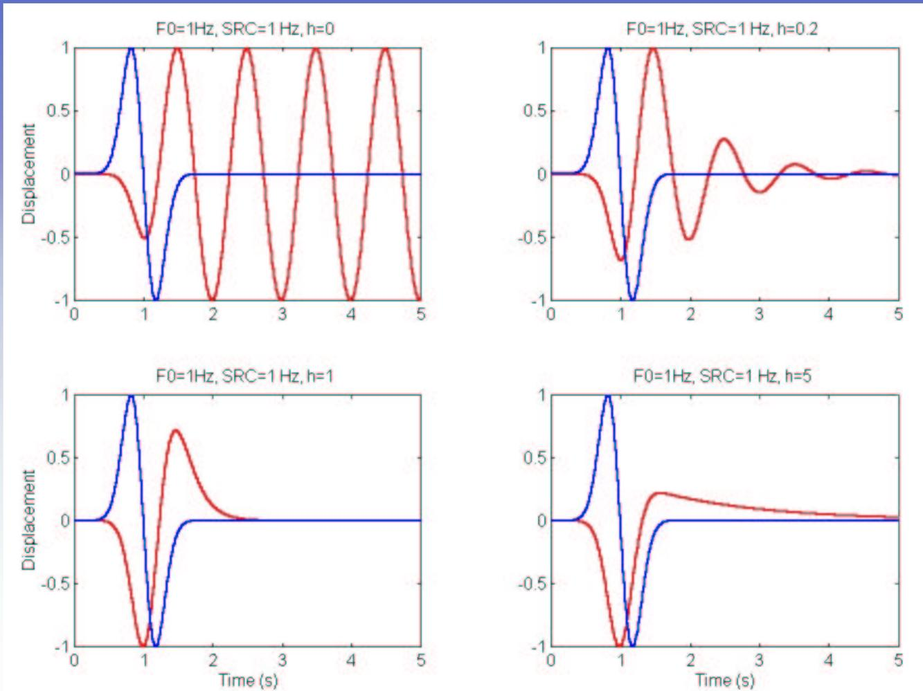
Ground motion (blue) – seismometer mass (red)
