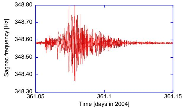
**Fig. 8.** The raw rotation measurement of the mag. 9.3 Sumatra earthquake from December 26, 2004. The dataset was recorded with a good signal to noise ratio.
