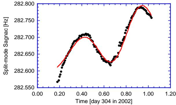
**Fig. 2.** Area strain for the UG1 ring laser location computed from a global model extended with a linear drift from atmospheric pressure changes (solid curve) superimposed on FSR measurements of the ring laser cavity (dotted curve).
