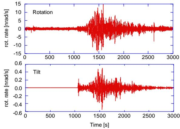
**Fig. 4.** Ring laser seismogram of an earthquake in Algeria (mag. 6.8) from May 21, 2003, recorded by the G ring laser in Wettzell. The tilt induced contribution to the measurement quantity is as large as 5%.
