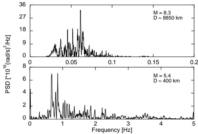
**Fig. 6.** Comparison of recorded rotation spectra from an teleseismic event (Hokkaido: Sept. 9, 2003) and a regional earthquake (France: Feb. 22, 2003). The much higher bandwidth of the rotational wave spectra requires alternative data acquisition techniques such as the demodulator.
