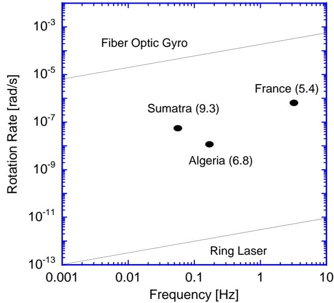
**Fig. 7.** Sensor resolution of different rotation sensor concepts in relation to the observed signal strength of some earthquakes at different epicentral distances.
