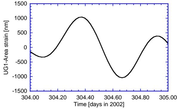
**Fig. 1.** Area strain for the UG1 ring laser location computed from global model for the day 304 in 2002. The maximum peak to peak variation of the perimeter is around  $2.5\mu\text{m}$ .
