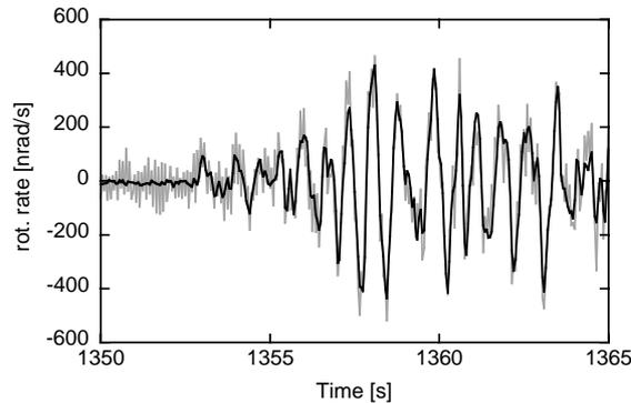
**Fig. 5.** Comparison of two ring laser seismograms from the the same mag 7.7 earthquake near Fiji on August 19, 2002. Both ring lasers were located in the same place with identical orientation. Apart from the higher noise level of the smaller instrument the recordings are identical.
