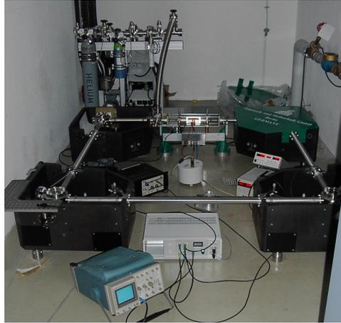
**Fig. 9.** Foto of the GEOsensor ring laser during sensor integration.
