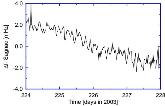
**Fig. 3.** Example of a timeseries of the Sagnac frequency variations from UG1. There is a general sensor drift apparent, but strain related scale factor changes are not present.
