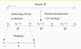
In order to facilitate the calculation of the space-dependent integrals we transform each element onto the standard interval [-1,1], illustrated here for  $n_e = 3$  elements. The elements share the boundary points.
