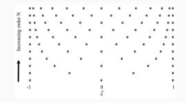
Illustration of the spatial distribution of Gauss-Lobatto-Legendre points in the interval [-1,1] from top to bottom for polynomial order 2 to 12 (from left to right). Note the increasing difference of largest to smallest interval between collocation points! Consequences?
