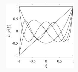
The Legendre polynomials are used to calculate the first derivatives of the Legendre polynomials. They can also be used to calculate the integration weights of the GLL quadrature.
