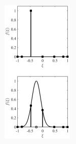
Top: A point-source polynomial representation (solid line) of a  $\delta$ -function (red bar). **Bottom:** A finite-source polynomial representation (solid line) as a superposition of point sources injected at some collocation points. For comparison with analytical solutions it is important to note that the spatial source function actually simulated is the polynomial representation of the (sum over)  $\delta$ -function(s).
