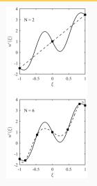
The function to be approximated is given by the solid lines. The approximation is given by the dashed line exactly interpolating the function at the GLL points (squares). **Top:** Order N = 2 with three grid points. **Bottom:** Order N = 6 with seven grid points.
