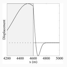
Detail of the finite-element simulation with varying element size at one of the domain boundaries. The crosses indicate the element boundaries and the changing element size. Note the continuous but non-differentiable behaviour of the displacement field at the interface.
