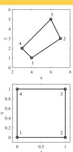
Quadrilateral elements. Mapping of physical coordinates (x,y, top) to a local reference frame (bottom) with coordinates  $\xi,\eta$ .
