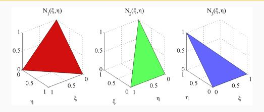
Triangular elements. The three corner nodes lead to an equivalent number of shape functions  $N_i(\xi, \eta)$  with unit value at one of the corners.
