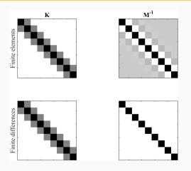
The structure of the system matrices for the finite-element method are compared with the finite-difference method formulated with matrix-vector operations. **Top row:** Stiffness and inverse mass matrix for the finite element method. **Bottom row:** Stiffness (differential) matrix and diagonal
