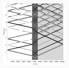
Snapshots of displacement values are shown as a function time. Where displacement amplitudes are below a threshold, the velocity models is shown in gray scale. Note the polarity change of the reflections at the boundaries and the slope of the signals in the x-t plane indicated their velocities.
