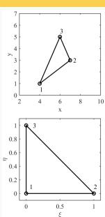
Triangular elements. Mapping of physical coordinates (x, y, top) to a local reference frame (bottom) with coordinates  $\xi, \eta$ .
