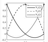
The sum over the weighted shape function of general order N gives the approximate *continuous* representation of the solution field  $u(\xi)$  inside the element.
