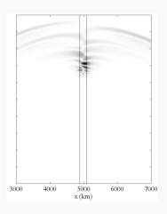
Snapshot of pressure amplitude for a source located at the left edge of a fault zone model
