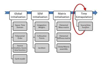
A substantial part consists of preparing the interpolation and integration procedures required to initialize the global mass- and stiffness matrices. The final time-extrapolation is extremely compact and does not require the inversion of a global matrix as is the case in classic finite-element methods.
