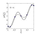
The function to be approximated is given by the solid lines. The approximation is given by the dashed line exactly interpolating the function at the GLL points (squares). **Top:** Order N = 2 with three grid points. **Bottom:** Order N = 6 with seven grid points.
