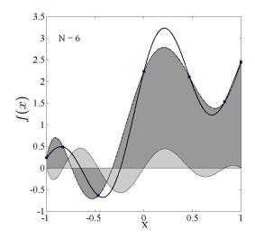
The exact function (thick solid line) is approximated by a Lagrange polynomials (thin solid line) that can be integrated analytically. Thus, the integral of the true function (thick solid) is replaced by an integral over the polynomial function (dark gray). The difference between the true and approximate function is given in light gray.
