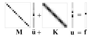
The unknown vector of coefficients  $\mathbf{u}$  is found by a simple finite-difference procedure. The solution requires the inversion of mass matrix  $\mathbf{M}$  which is trivial as it is diagonal. That is the key feature of the spectral element method.
