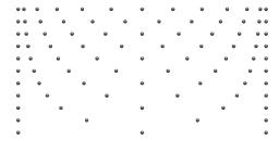
Illustration of the spatial distribution of Gauss-Lobatto-Legendre points in the interval [-1,1] from top to bottom for polynomial order 2 to 12 (from left to right). Note the increasing difference of largest to smallest interval between collocation points! Consequences?
