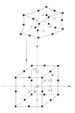
In 3D elements might be skewed and have curved boundaries. The calculation of the Jacobian is then carried out analytically by means of shape functions.
