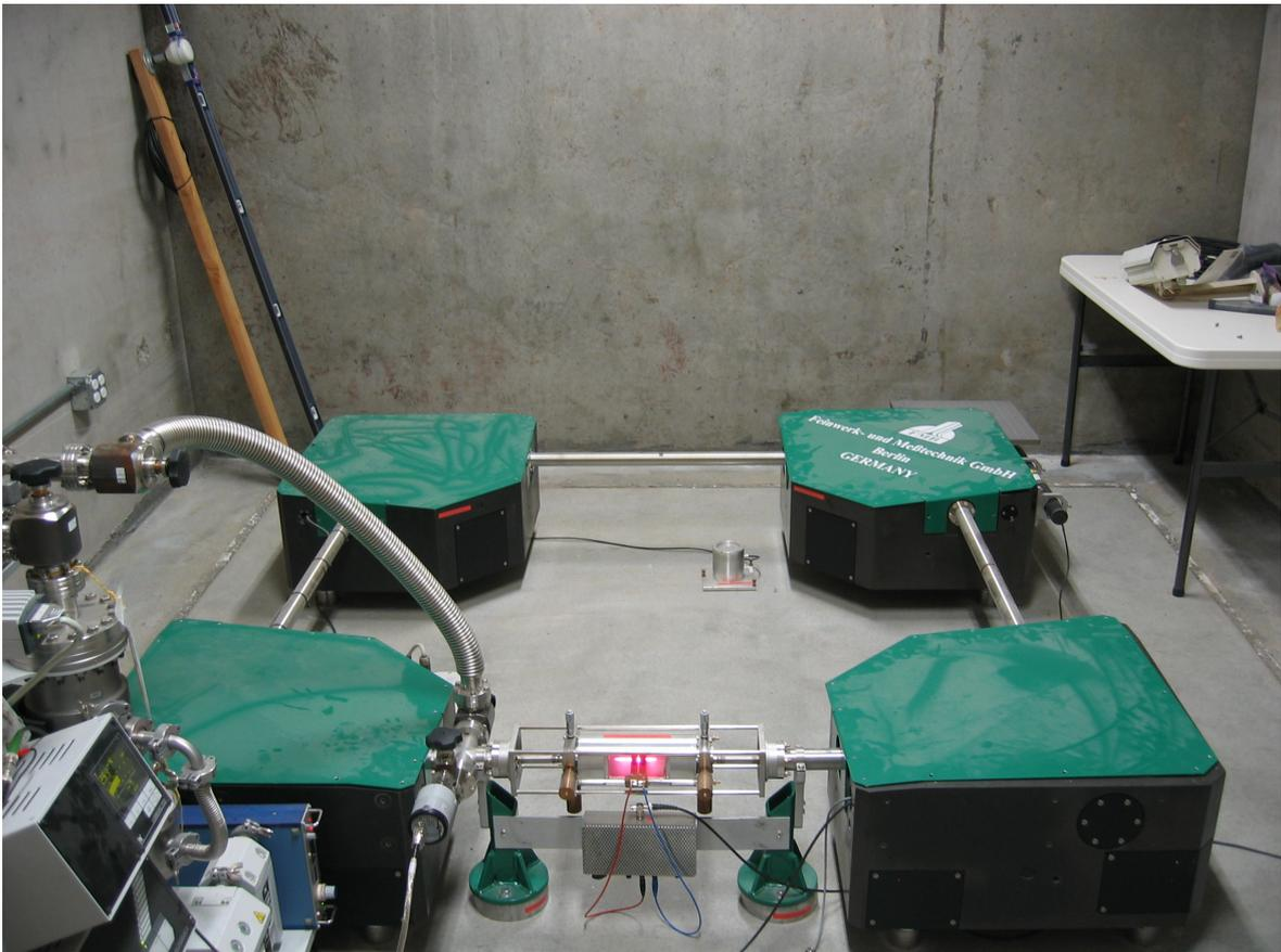
Figure 3.15.: This picture shows the operable ring laser component of the GEOsensor with the gain tube in front (middle), the four cornerboxes (with the mirror holders inside) and the tiltmeter (in the back).
