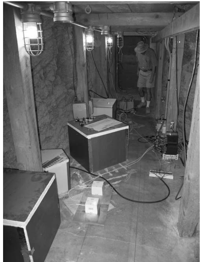
Figure 3. Seismic monitoring tunnel at ASL. Two R-1s are on the floor undergoing noise testing. Other covered instruments are reference broadband seismometers. The Q330 digitizers are on the floor to the right.
