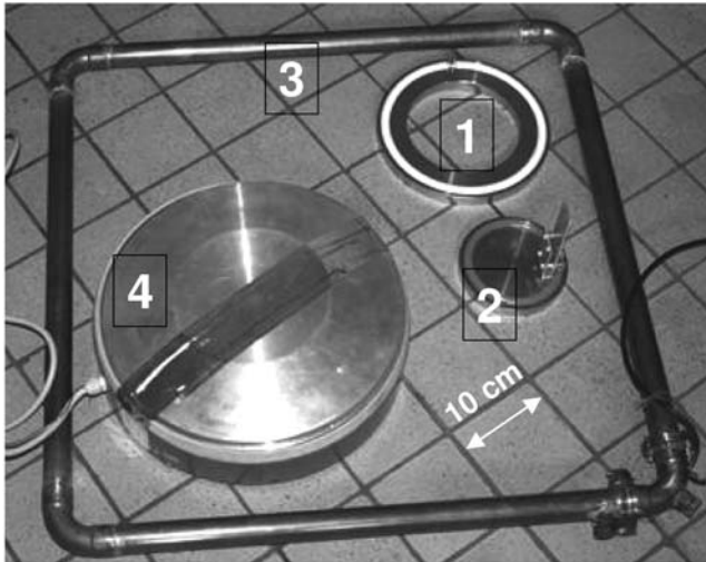
Figure 4. Samples of technical variants of tested fluid rotational seismometer tubes. 1, 2: one-ring parts of rotation seismometer (ring diameters 200 mm and 110 mm, respectively), 3: square-shaped metal tube of rotational seismometer of diameter 600 mm, 4: multiring tube part of rotation seismometer of diameter 300 mm, n = 30 , and inner tube diameter 8 mm.
