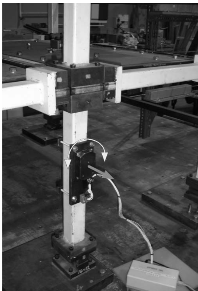
Figure 6. View of the installation of the FOG on the building model on the shake table.
