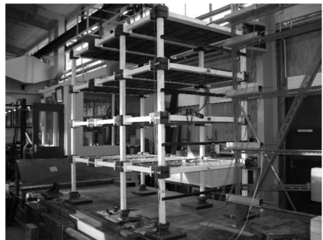
Figure 5. View of the shake table with a four-story model mounted on top. Reaching in from the right-hand side one can see five displacement transducers mounted on a reference frame fixed to the laboratory floor.
