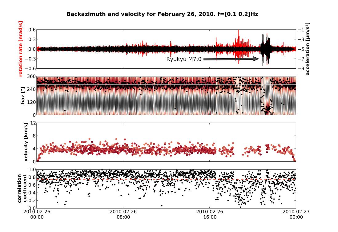
(a) Rotation rate (red), transverse acceleration (black). Event (M<sub>W</sub>7.0 Ryukyu) with backazimuth = 45°. (b) Backazimuth, colorscale is the cross-correlation coefficient (red: positive high; black: negative high). (c) Phase velocity obtained from amplitude ratio  $\left(\frac{a_T}{\dot{\omega}_z}\right)$ . (d) Maximum correlation coefficient. f = [0.1 0.2]Hz
