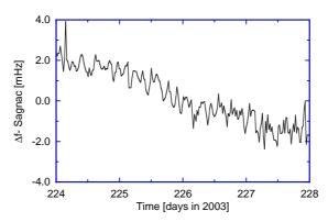
**Fig. 3.** Example of a timeseries of the Sagnac frequency variations from UG1. There is a general sensor drift apparent, but strain related scale factor changes are not present.
