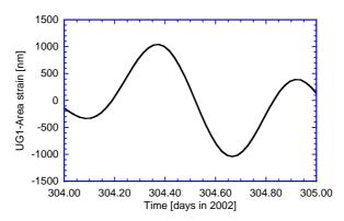
Fig. 1. Area strain for the UG1 ring laser location computed from global model for the day 304 in 2002. The maximum peak to peak variation of the perimeter is around  $2.5\mu m$ .
