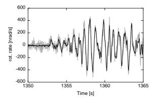
**Fig. 5.** Comparison of two ring laser seismogramms from the the same mag 7.7 earthquake near Fiji on August 19, 2002. Both ring lasers were located in the same place with identical orientation. Apart from the higher noise level of the smaller instrument the recordings are identical.
