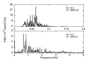
**Fig. 6.** Comparison of recorded rotation spectra from an teleseismic event (Hokkaido: Sept. 9, 2003) and a regional earthquake (France: Feb. 22, 2003). The much higher bandwidth of the rotational wave spectra requires alternative data acquisition techniques such as the demodulator.
