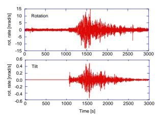
**Fig. 4.** Ring laser seismogram of an earthquake in Algeria (mag. 6.8) from May 21, 2003, recorded by the G ring laser in Wettzell. The tilt induced contribution to the measurement quantity is as large as 5%.
