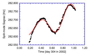
**Fig. 2.** Area strain for the UG1 ring laser location computed from a global model extended with a linear drift from atomspheric pressure changes (solid curve) superimposed on FSR measurements of the ring laser cavity (dotted curve).
