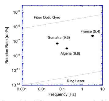
**Fig. 7.** Sensor resolution of different rotation sensor concepts in relation to the observed signal strength of some earthquakes at different epicentral distances.
