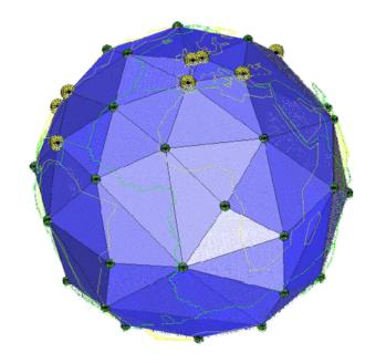
Gridding of a spherical surface used in FE modelling of the Earth's magnetic field. (From A. Schultz, Cambridge)
