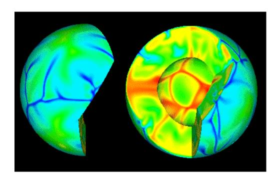
Thermal convection is modelled in 3-D a finite-element technique. The mesh has about 10 million grid points. From Peter Bunge, Princeton.
