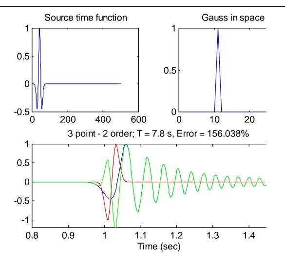
Example of acoustic 1D wave simulation. FD 3 -point operator red-analytic; blue-numerical; green-difference
