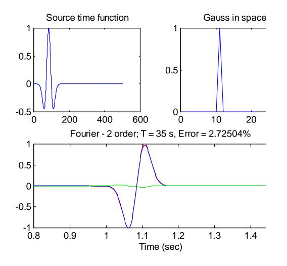
Example of acoustic 1D wave simulation. Fourier operator red-analytic; blue-numerical; green-difference
