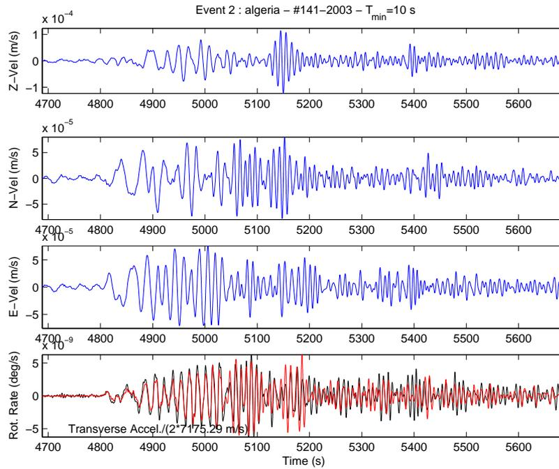
**Fig. 10.** Three components of translations (blue) and comparisons of transverse acceleration (black) and rotation rate (red) for one example in the event data base (superimposed traces at the bottom). Note the consistent match for most of the seismogram except towards the end where scattering may lead to phases arriving from out-of-plane directions. Conversion phase velocities are given in the lower left corner.
