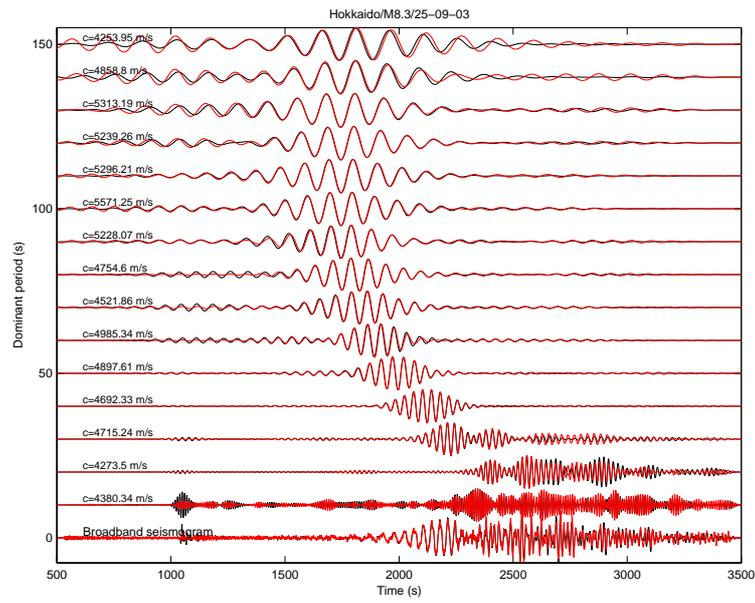
**Fig. 12.** Frequency dependent comparison of rotations (red) and accelerations (black). The vertical axis is central period of a very narrow band-pass filter. Note the excellent match at periods down to 150 s. Note also the general increase in best-matching phase velocities as expected from theoretical Love-wave dispersion.
