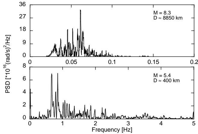
**Fig. 7.** Comparison of recorded rotation spectra from an teleseismic event (Hokkaido: Sept. 9, 2003) and a regional earthquake (France: Feb. 22, 2003). The much higher bandwidth of the rotational wave spectra requires data acquisition techniques such as the demodulator
