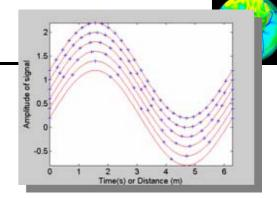
The frequency half of the sampling rate dt is called the Nyquist frequency  $f_N=1/(2dt)$ . The distortion of a physical signal higher than the Nyquist frequency is called aliasing.
