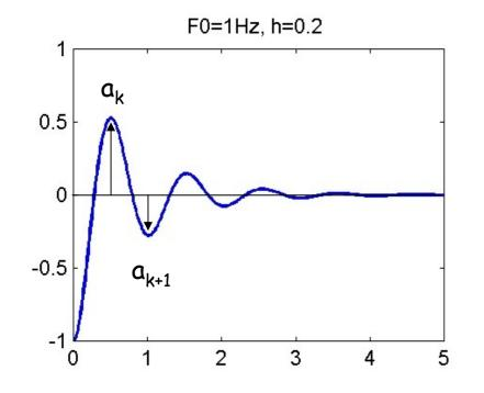
The damping coefficients can be determined from the amplitudes of consecutive extrema  $a_k$ and  $a_{k+1}$ We need the logarithmic decrement  $\Lambda$
