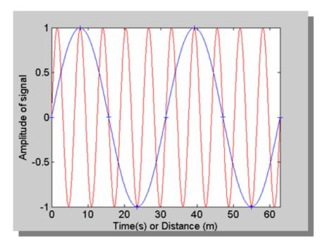
The frequency of the physical signal is  $> f_N$  is sampled with (+) leading to the erroneous blue oscillation.
