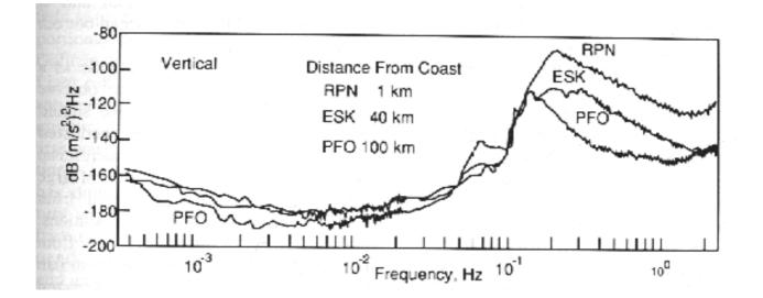
Observed seismic noise as a function of frequency (power spectrum). Note the peak at 0.2 Hz and decrease as a distant from coast.
