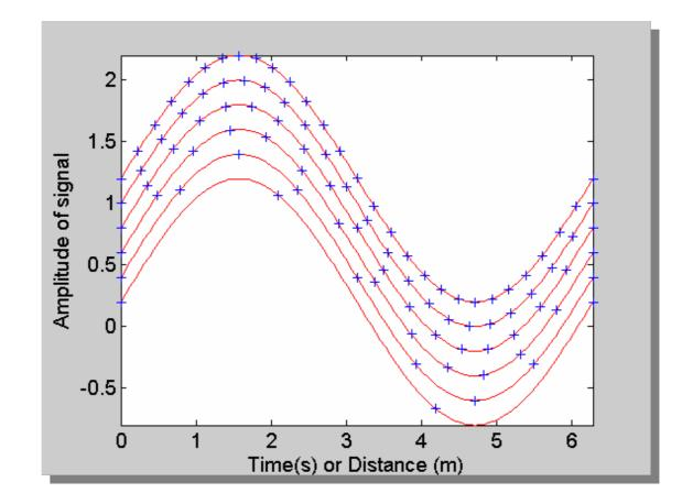
Sampling frequency, sampling rate is the number of sampling points per unit distance or unit time. Examples?
