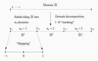
In order to facilitate the calculation of the space-dependent integrals we transform each element onto the standard interval [-1,1], illustrated here for  $n_e = 3$  elements. The elements share the boundary points.
