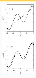
The function to be approximated is given by the solid lines. The approximation is given by the dashed line exactly interpolating the function at the GLL points (squares). **Top:** Order N = 2 with three grid points. **Bottom:** Order N = 6 with seven grid points.
