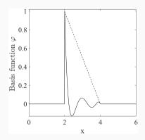
Illustration of local basis functions. By defining basis functions only inside elements the integrals can be evaluated in a local coordinate system. The graph assumes three elements of length two. A finite-element type linear basis function (dashed line) is shown along side a spectral-element type Lagrange polynomial basis function of degree N=5 (solid line).
