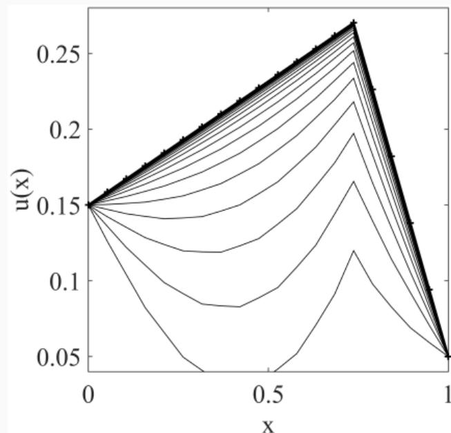
Simulation example comparing the finite-element solution (thick solid line) with a finite-difference based relaxation method (thin lines) that iteratively converges to the correct solution (see text for details). 500 iterations were employed for the relaxation method and the solution is shown after any 25 iterations.
