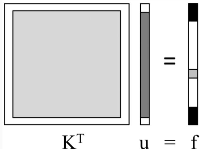
Graphical representation of the matrix-vector system with boundary conditions. The global system matrix has  $N-2 \times N-2$  elements. The system *feels* the boundary conditions through a modified source terms. The red spot indicates the source location inside the medium.
