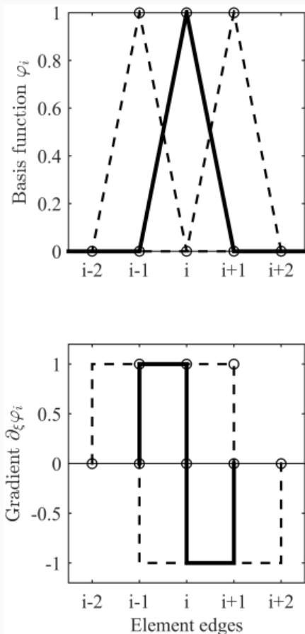
Basis functions and their derivatives. **Top:** The basis function  $\varphi_i$  (thick solid line) is shown along with the neighboring functions  $\varphi_{i\pm 1}$  (thin dotted lines). **Bottom:** The same for their derivatives with respect to the space coordinate  $\xi$ .
