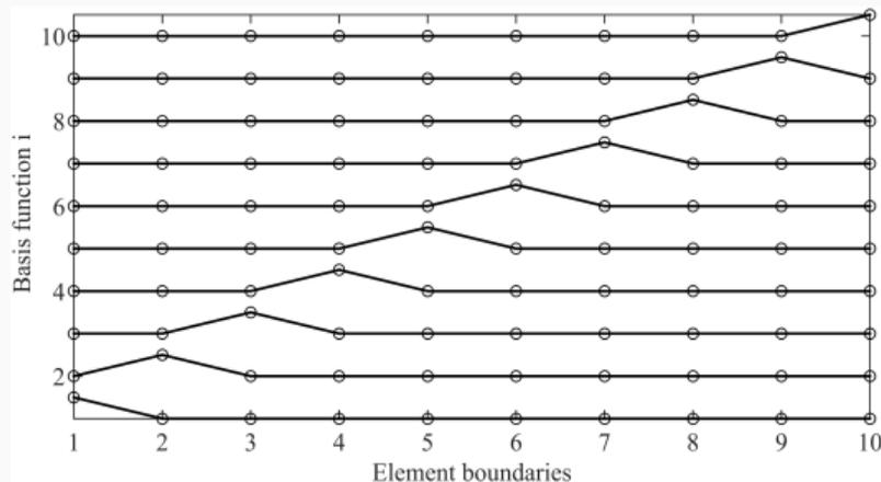
Linear basis functions for the finite-element method. A 1D domain is discretized with  $n - 1$  elements having  $n = 10$  element boundaries (open circles). The basis functions  $\varphi_i = 1$  at  $x = x_i$ . With this basis an arbitrary function can be exactly interpolated at the element boundary points  $x_i$ .
