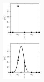
Top: A point-source polynomial representation (solid line) of a  $\delta$ -function (red bar). **Bottom:** A finite-source polynomial representation (solid line) as a superposition of point sources injected at some collocation points. For comparison with analytical solutions it is important to note that the spatial source function actually simulated is the polynomial representation of the (sum over)  $\delta$ -function(s).
