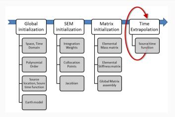
A substantial part consists of preparing the interpolation and integration procedures required to initialize the global mass- and stiffness matrices. The final time-extrapolation is extremely compact and does not require the inversion of a global matrix as is the case in classic finite-element methods.
