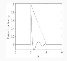
Illustration of local basis functions. By defining basis functions only inside elements the integrals can be evaluated in a local coordinate system. The graph assumes three elements of length two. A finite-element type linear basis function (dashed line) is shown along side a spectral-element type Lagrange polynomial basis function of degree N=5 (solid line).
