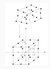
In 3D elements might be skewed and have curved boundaries. The calculation of the Jacobian is then carried out analytically by means of shape functions.
