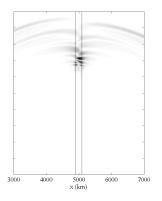
Snapshot of pressure amplitude for a source located at the left edge of a fault zone model It indicates the occurence of head waves and the development of a dispersive wavefield trapped inside the low-velocity zone
