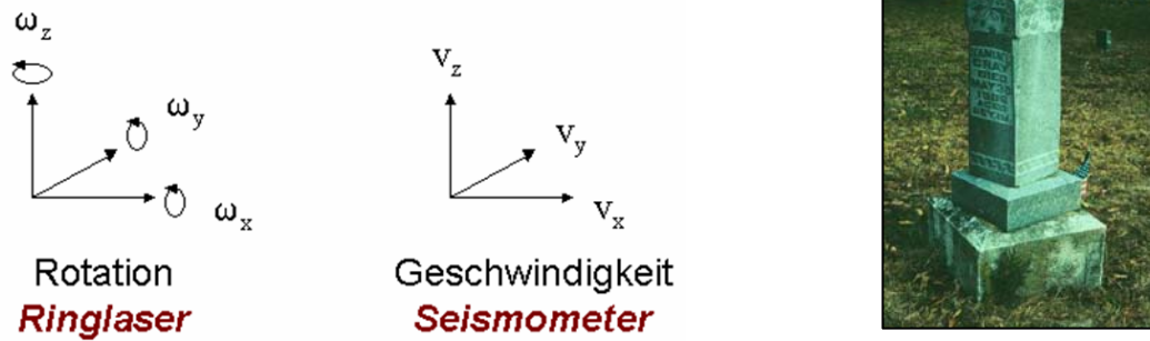
Fig. 1. Left: Three components of rotational motions that can be measured with rotation sensors as well as three components of translations measured with standard seismometers. Right: Rotation of a symmetric structure that is difficult to explain with pure translational motions. Rotational accelerations are thought to cause such effects.
